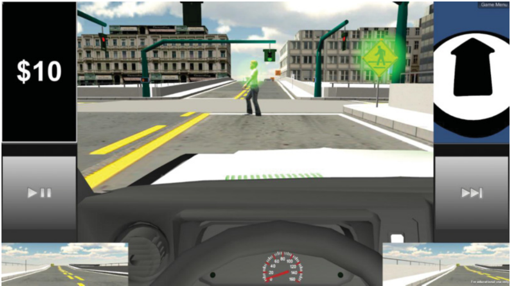
Fig. 6. Example of ROI highlighting after a gaze-related trial failure. Both the male pedestrian and the pedestrian crossing sign have become highlighted with a green light to draw the attention of the driver.
